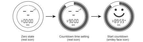
Zero state (rest icon) Countdown time setting (rest icon) Start countdown (smiley face icon)
